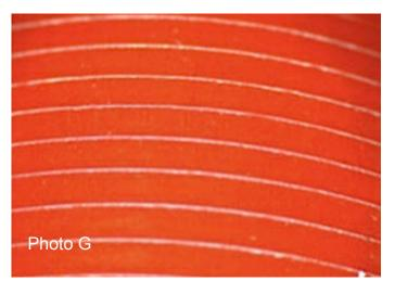
The purpose of the binding is to create pressure that will force the resin and the carbonfibres to all bond as one when they go into the oven to be 'cooked' at really high temperatures. The resultant behaviour of the pole is affected by the pressure of the winding, the pressure in the oven, the temperature of the oven, and the time in the oven.
