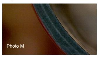
(M) Red outer layer... and you can see the telling sign of two layers of fibreglass in the carbonfibre pole.
