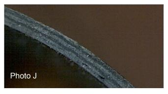
(J) A Hybrid Pole - this design uses alternate layers of fibreglass and carbonfibre.
