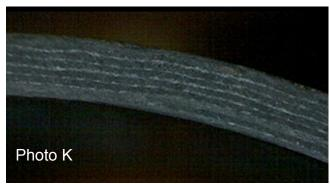
(K) A High Modulus Carbonfibre. Each layer is clearly marked by the ultra fine membrane that backs the high-tech prepreg and assists the spread of the resin throughout the fibres.
