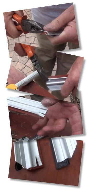
Again, I decided to sit down and really think about this. It was then that I noticed that if the rubber blade were cut closer to the edge of the channel then this would marginally improve things along with the dog-earing. Having done this I noticed that the rubber *above* and on top of the channel was longer and it seemed to me that *this* could be the problem. But what could be done?
